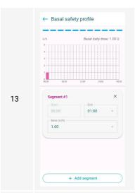
Enter your basal safety profile: start time, end time and desired rate per hour for each time slot. One time slot can cover several hours. The maximum number of slots is 24. When loop mode is off, the DBLG2 system switches to this basal safety treatment.
